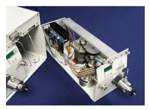
The Pump mechanism, Control Boards, & Pulse Dampener (with Pressure Transducer) are accessible by removing pump drawer.
